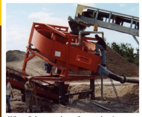
When fed a wet slurry from a density separator or hydrocyclone, the ORTNER may be used to dewater, classify, or remove excess fines from the slurry.
